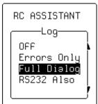
Turn to— Scroll Log Push to Clear Used for monitoring remote commands received through the GPIB and RS-232 remote control ports, the Remote Control Assistant helps debug communications between the oscilloscope and the PC. When activated, it displays a log of the dialog taking place through the remote control ports of the oscilloscope. When a communication error occurs, RC Assistant gives the additional message "Remote Control: problem detected and logged."
