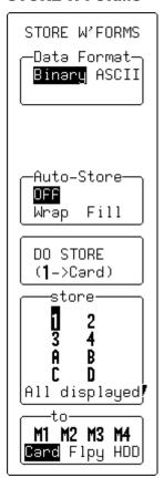
Press WAVEFORM to store waveforms to internal memory (M1, M2, M3, or M4) in LeCroy's binary format. You can also store waveforms in binary or ASCII format on floppy disk, memory card, or removable hard disk (HDD) where available.
